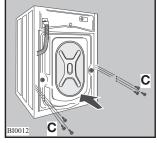
Fill the smaller upper hole and the two large ones with the corresponding plastic plug caps supplied in the bag containing the instruction booklet that you will find inside the drum.
